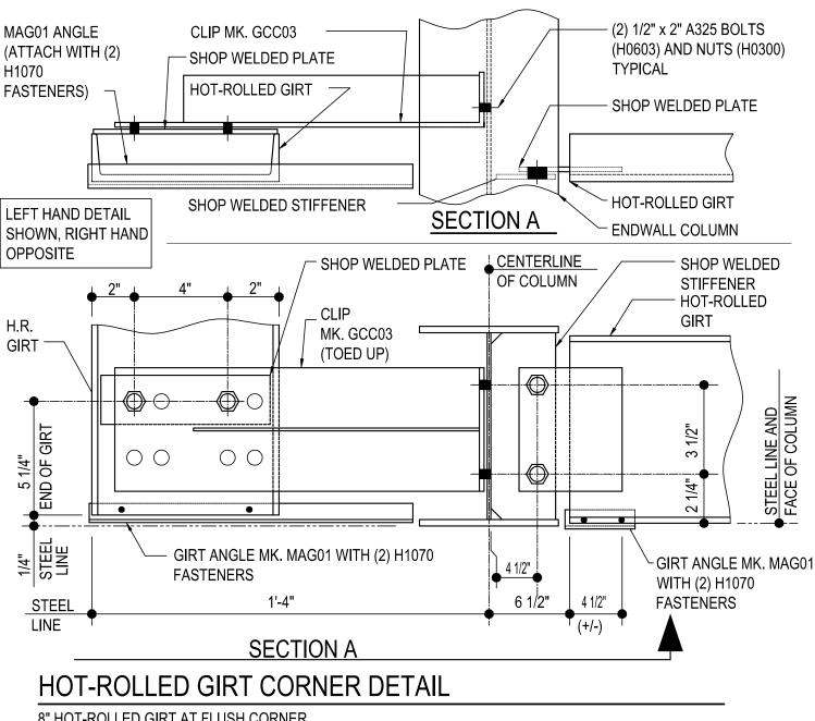
8" HOT-ROLLED GIRT AT FLUSH CORNER. NOTE: USE (6) 1/2" x 2" A325 BOLTS (MK. H0603) & NUTS (MK. H0300) REFERENCE ERECTOR NOTE FOR TYPCIAL WASHER REQUIREMENTS
