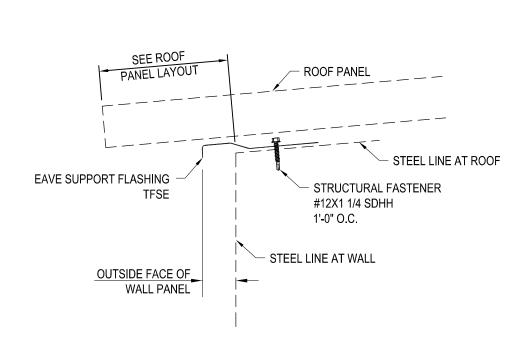
NOTE: EAVE SUPPORT FLASHING NOT REQUIRED AT LONG SPAN III ROOFS.
