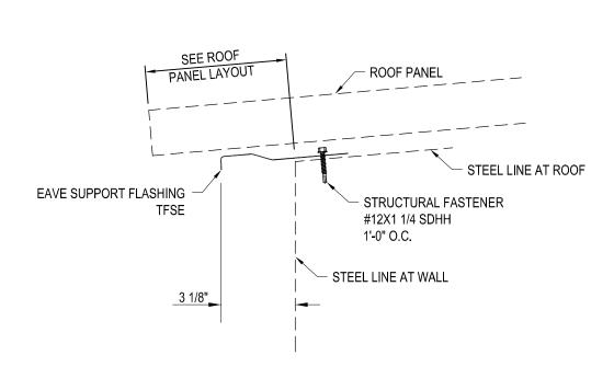
NOTE: EAVE SUPPORT FLASHING NOT REQUIRED AT LONG SPAN III ROOFS.
