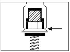
3. The base of the nut setter should now be contacting the top of the head of the fastener with no gaps.
