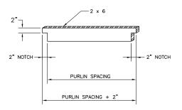
Straight purlins are a necessity. Zee sections have a natural tendency to roll out of plane and deflect horizontally. This must be corrected by forcing the purlins into proper plane and spacing. Wood blocking is recommended as one method to accomplish this.
