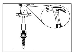
2. Place the point of the fastener onto a hard surface and firmly hit the top of the nut setter 2-3 times.
