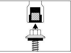
1. Put the top of the fastener into the nut setter. Note: for painted Fasteners, place a single or doubled layer of plastic between the fastener head and the nut setter.
